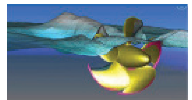
Figure 12. MSC Nastran - scFLOW prediction of propeller with free surface and cavitation
