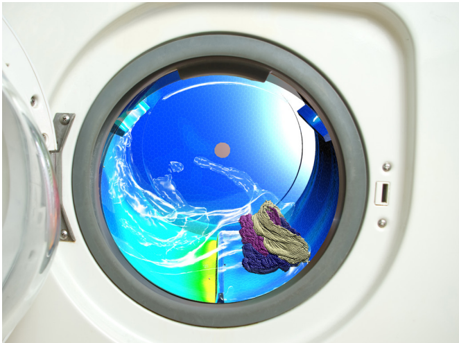
Combined fluid-structure-multibody interaction co-simulation of a washing machine drum using a Cradle CFD – Marc – Adams coupling.
